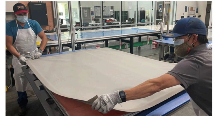
Boeing EnCore Interiors layup technicians Alberto Nieto Garcia (left) and Bang Nguyen laying out a silicone bag as part of the 737 floor panel fabrication process. The new reusable bagging system is expected to save an estimated $175,000 annually in material costs. (David Brink photo)
